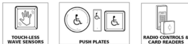
Figure 1 [11]: Varying types of interfaces for ADA door opening systems
